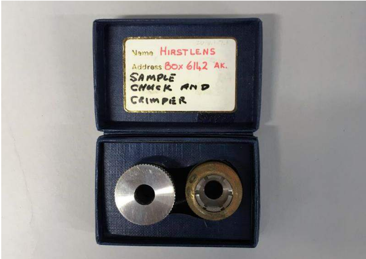
Astigmatic Lens Collet I designed in 1976 - the collet had two horizontally opposed tangs thicker than the rest and when pressure was applied by rotating the brass sleeve, a toroidal profile was induced into the plastic blank – the posterior curve was then cut into the crimped blank, polished and released to form a surface with two curves at 90° with each other and therefore two focal lengths. The degree to which the brass collet was turned determined the difference in surface geometry.
