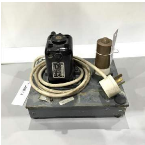
A miniature drill used to fenestrate contact lenses
