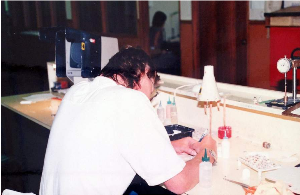
Polishing a contoured edge on the lens – note the thickness gauge on the shelf and the strips of Leukoplast hanging from the lamp shade!
