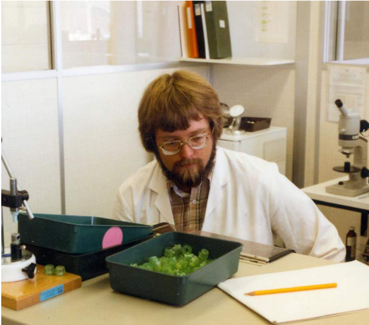
Developing the mounting system – the green modules were the prototype disposable collets (see also below)
