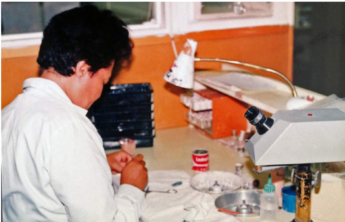
Polishing lenses - note the Leukoplast and bottle of pink Silvo (just to the right of the green-top bottle of iso-propyl alcohol [dry cleaning fluid!]) and the spindles mounted in the bench inside inverted aluminium jelly moulds – we were the masters of adaptation!
