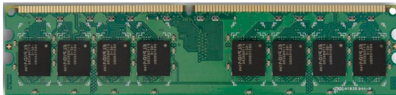
RAM (Random Access Memory - older generation) - storing the data and programs your CPU is actively using
