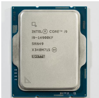
CPU (central processing unit) - serves as the brains behind a PC's operation
